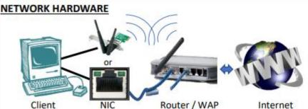
All clients need an NIC to connect to a ROUTER. This could be a wireless adapter or a network card.
